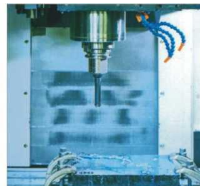
CNC 数控机床，中低速钻削时请选择粉末高速钢系列，高速钻削时请选择硬质合金系列。 CNC machine tools, medium and low speed drilling please choose powder high speed steel series, please choose carbide series when high-speed drilling.
